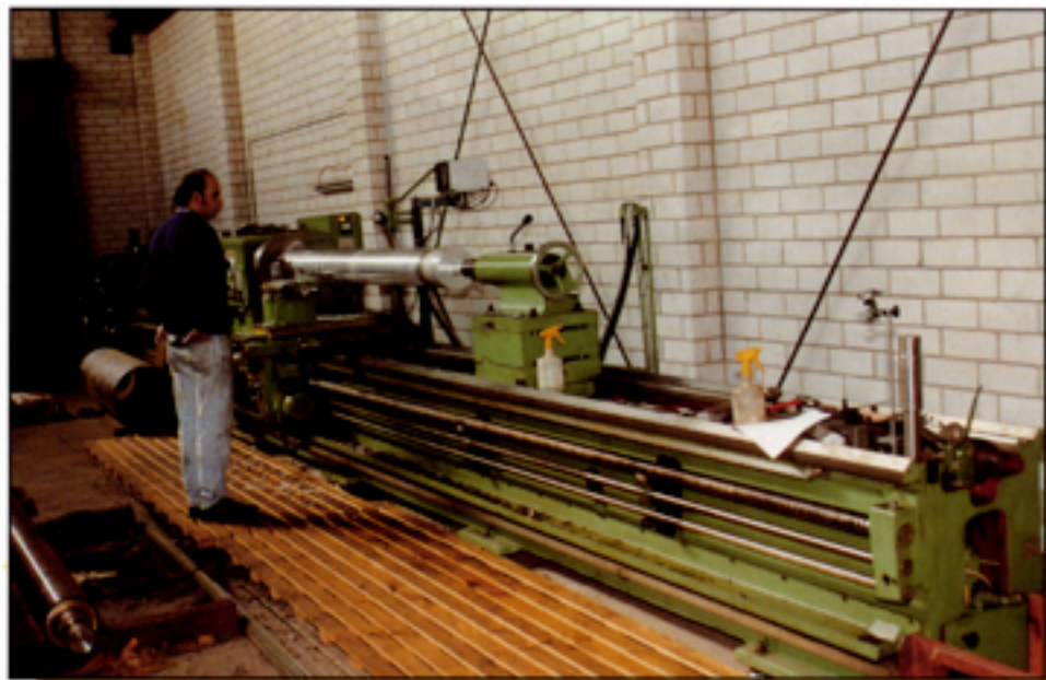
➤ Ø 200 x 2500 mm Aluminium Roller in the Course of Machining
